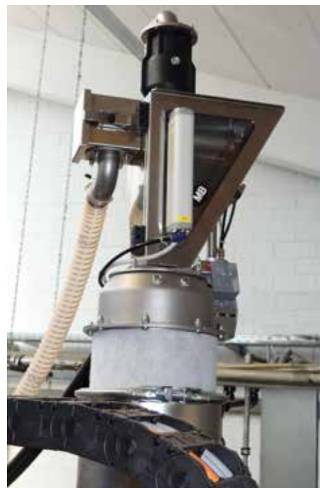
Fig. 4. TS5 sifter module used in production at neo-plastic for dedusting PMMA granulate (© Ingenieurbüro Fischer)
