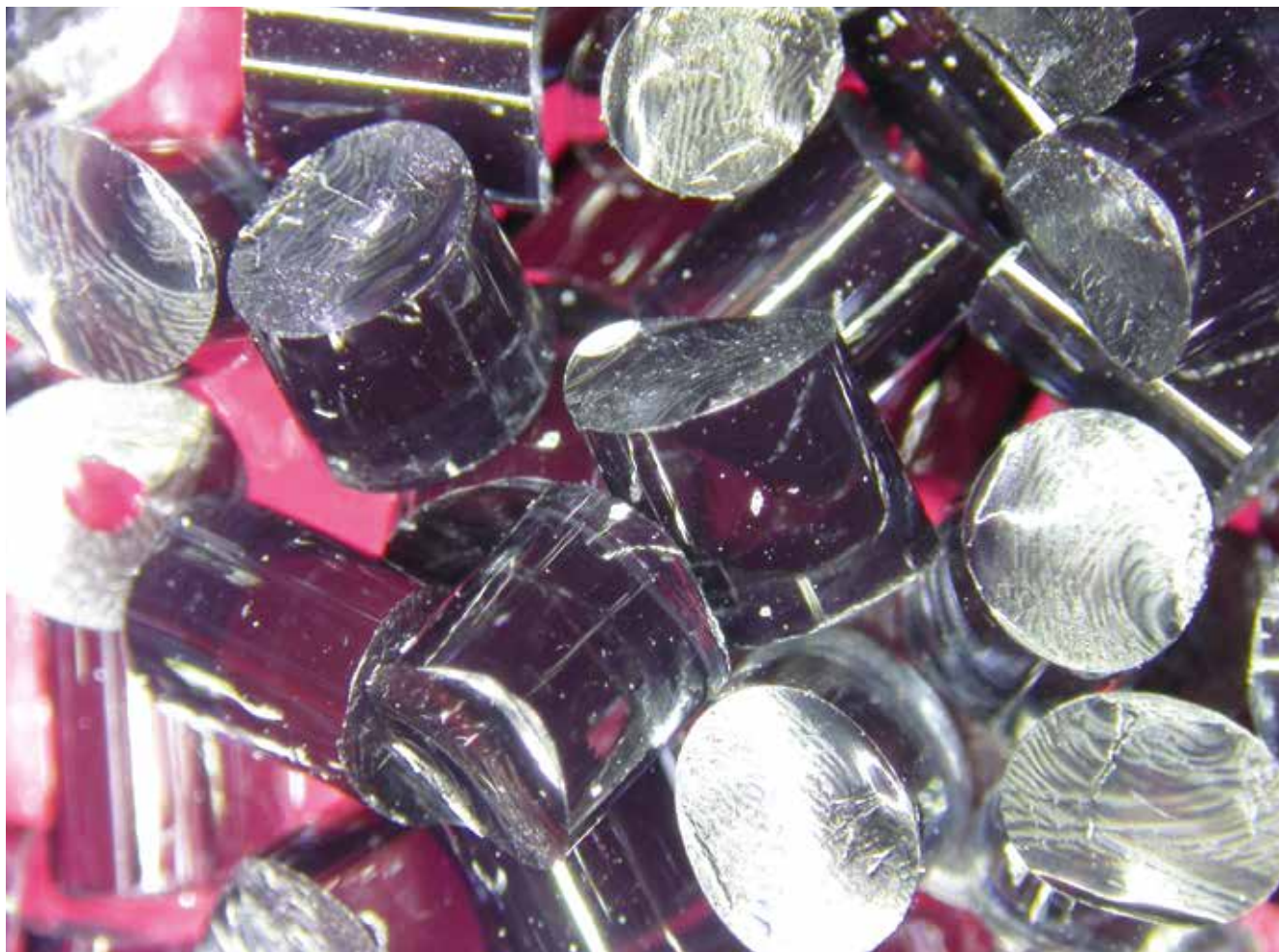
PMMA granulate with polymer dust sticking to it (© neo-plastic)
