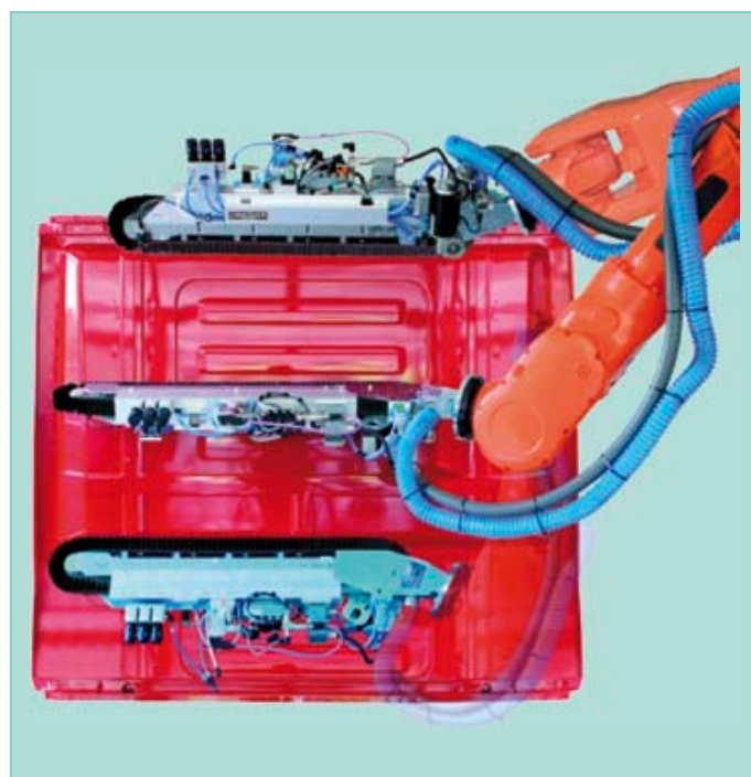
Fig. 2: Sword brushes guided by a robot (Source: Wandres GmbH micro-cleaning)
