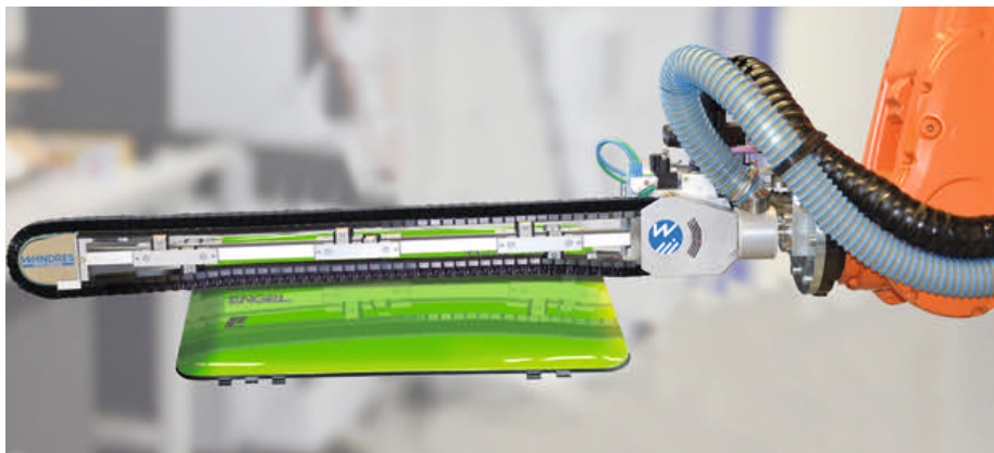
A current application from Engel: a sword brush removed particles from both sides of a back-molded lap-top cover before the latter is placed in the mold (figures: Wandres GmbH)
